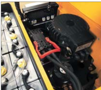
Drive and lift motor with AC technology
