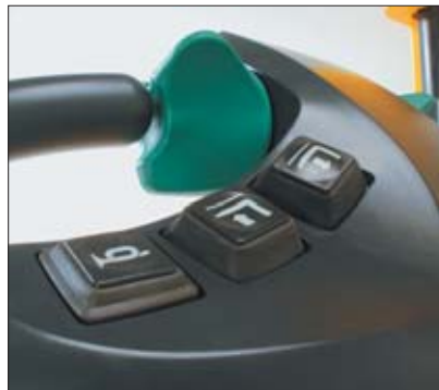
Buttons for sensitive lifting and lowering as well as horn
