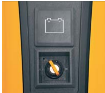
Combined discharge indicator with state of charge display
