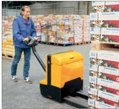
Collision protection on battery compartment
