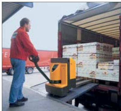
Travel stability with sprung support rollers
